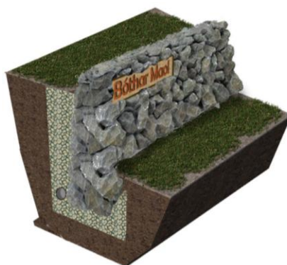
Figure 2-8 Cross Section of a 'Louth Wall' (Extract from Park Hood Drawing Pack, Drg. No. L2107 , Park Hood)
